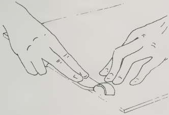
Position of the arm and hand while skiving. —Modern Leather Design
